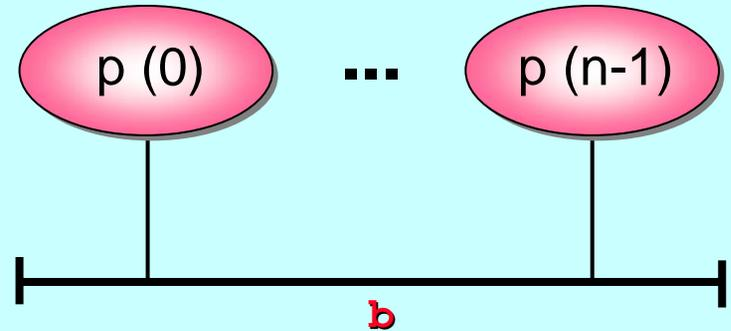
(d)  $n$  processes enrolled on a shared barrier (any process synchronising must wait for all to synchronise).
