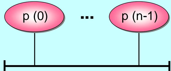
(d) n processes enrolled on a shared barrier (any process synchronising must wait for all to synchronise).
