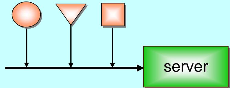
(b) three processes sharing the writing end of a channel to a server process.
