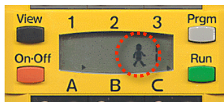
Figure 5. The ‘walking figure’ on the LCD display of the RCX
