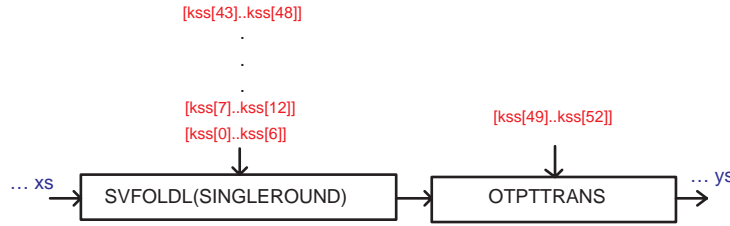
Figure 23: IDEA encryption block diagram in its second design with streamed input and output.
